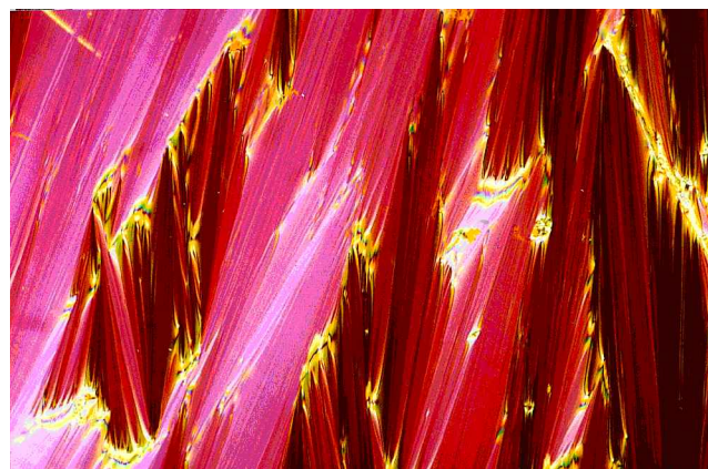
Figure 7. Texture photograph of DMS-3 at 115^\circ\text{C} (Sm2 phase). Comparing with figure 6 it can be seen that the bands disappear and focal-conics are sharpened ( \times 160 magnification).
